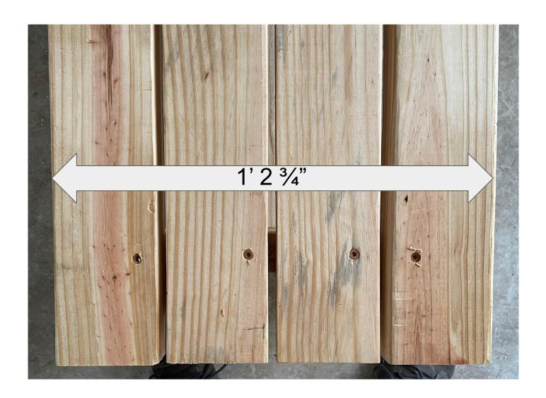
Once you secure the 2 end boards line up and overhang the middle boards 1  $\frac{1}{2}$ " off the side as well and space the boards evenly. If done correctly the benchtop should be 1' 2  $\frac{3}{4}$ " wide.
