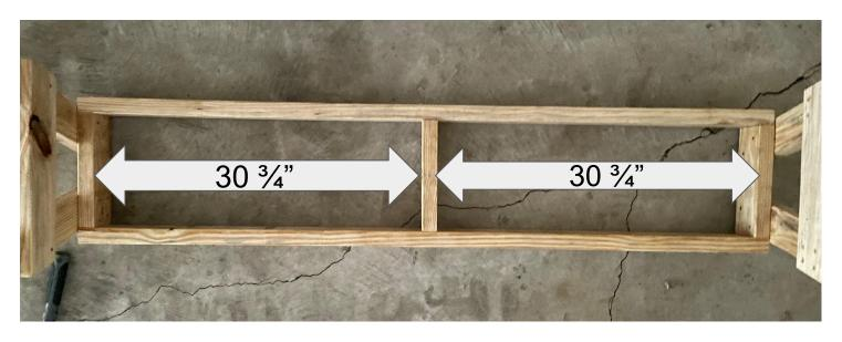
Install middle brace for the frame by setting the inside gap between it and the leg 30 <sup>3</sup>/<sub>4</sub>" apart. This will set the brace in the middle of the frame. Then attach by using 2 screws to secure it on each side.
