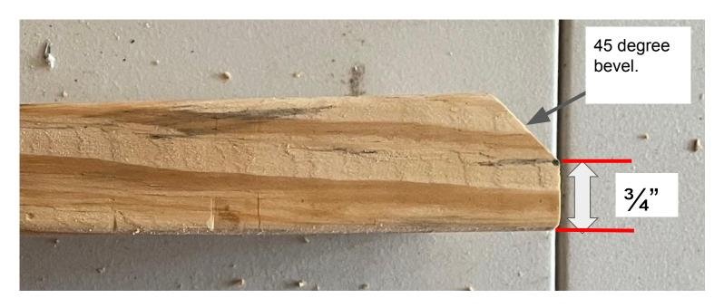
Once all pieces are cut we will make a chamfer bevel on both ends of each board according to the above dimensions.
