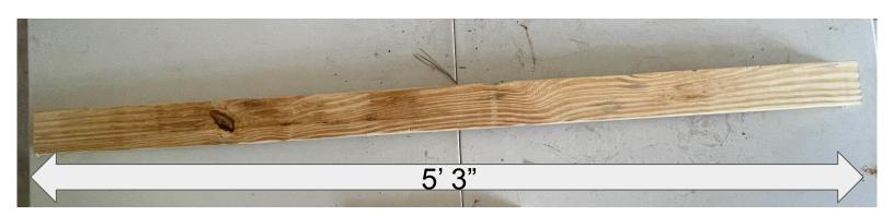
The final part of the bench frame is a brace that will attach to the 1'5" bottom braces on the legs. Cut 2-5' 3" pieces. One for each bench.
