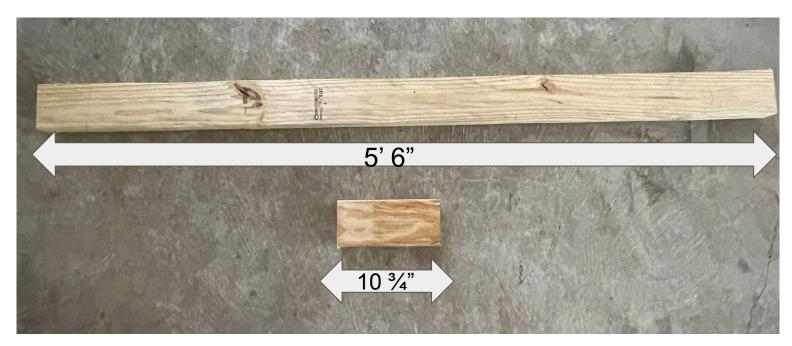
Next, cut the frame boards to attach the legs together for both benches. You will need to cut.
