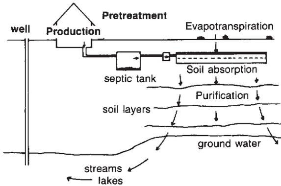
Figure 6. Soil Disposal of Septic Tank Effluent.
