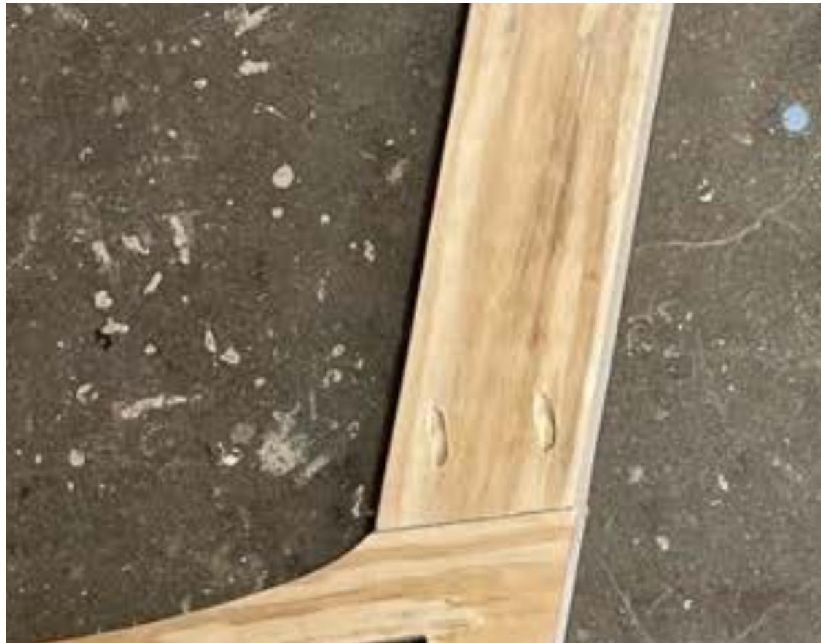
Next, align the back braces on the angled end of the seat braces and attach using 2 ½" screws.
