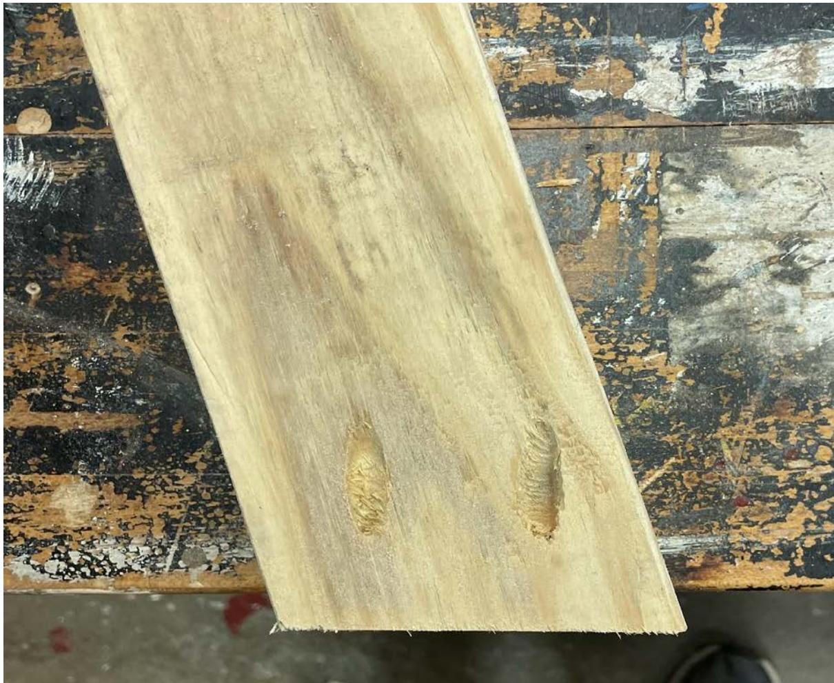
Using a pocket hole jig drill pocket holes for 2 screws on each 21" back brace. Two of the braces should have pocket holes on the right side of the board and 2 of the braces should have pocket holes on the left side of the braces. This way all pocket holes are facing toward the middle of the swing.
