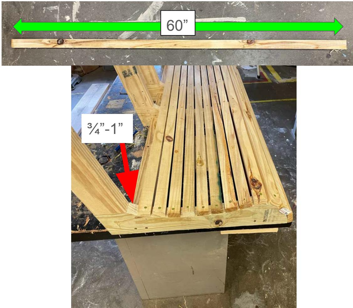
Take the pre-ripped 1x2s and cut twelve 60" pieces for the seat slats. Space the slats  $\frac{1}{4}$ ". You will end up with a  $\frac{3}{4}$ "-1" gap between the last slat and the back brace. Attach slats using  $1\frac{1}{2}$ " screws. Pre-drill holes for screws to avoid splitting the slats.
