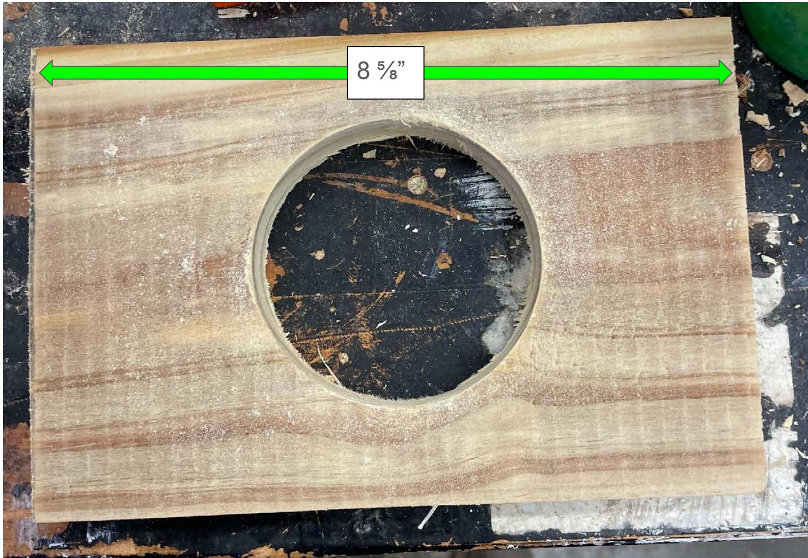
Cut from the 1x6 two  $8 \frac{5}{8}$ " pieces measure length and width to find the center of the board and cut a 3 in hole for the cup holder on both pieces.
