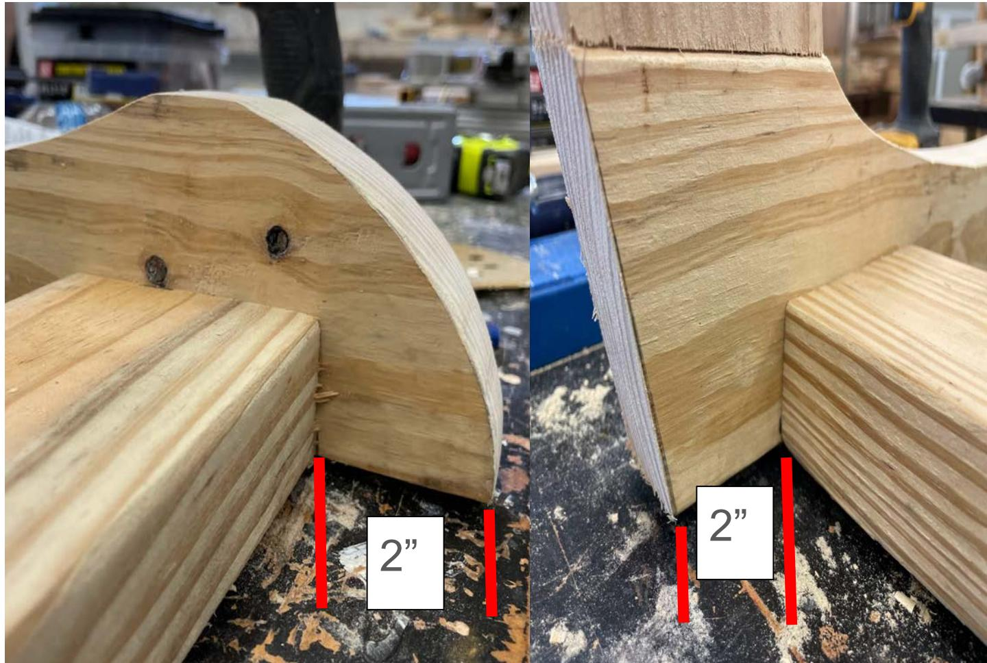
Attach the end braces to the two bottom cross braces position the cross braces 2" from the front of the seat braces and 2" from the bottom of the back of the seat brace.
