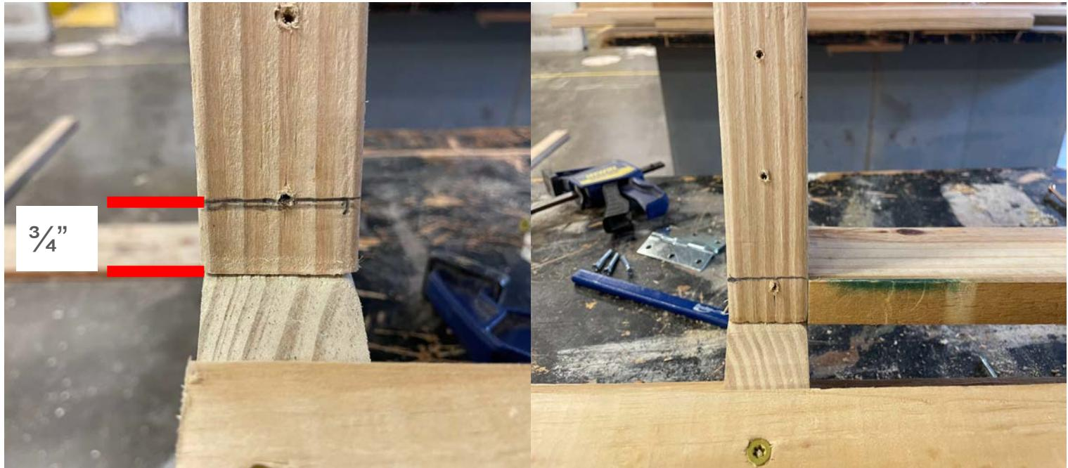
Mark a line on each back brace at  $\frac{3}{4}$ " from the joint with the seat brace.
