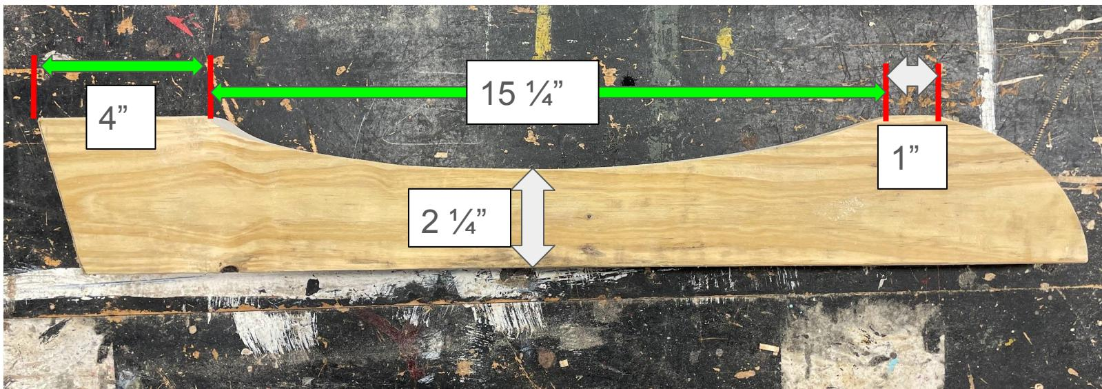
Come off the front curve of the 24" seat braces an inch and draw out a  $15 \frac{1}{4}$ " curve for the seat of the swing. The middle of the curve should be  $1 \frac{1}{4}$ " deep leaving  $2 \frac{1}{4}$ " of the original width of the brace. The seat should end leaving a 4" tail where the back braces will attach.
