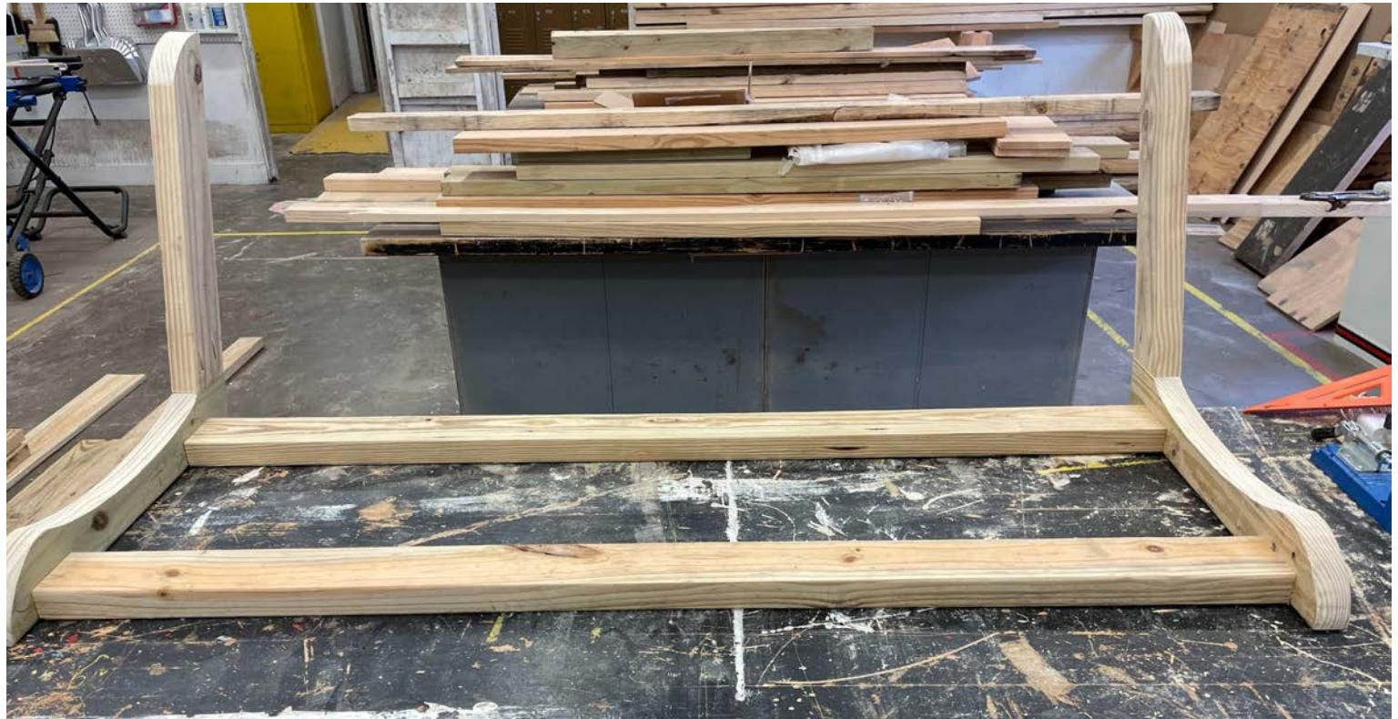
Once the outside braces and are screwed to the cross braces next will be to position the middle braces.
