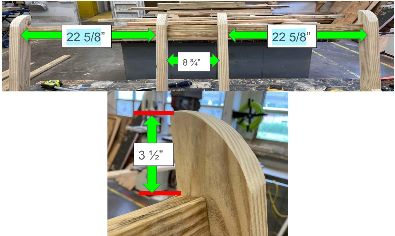
Insert the back cross brace then space and attach in the same manner as the seat using  $2 \frac{1}{2}$ " screws.
