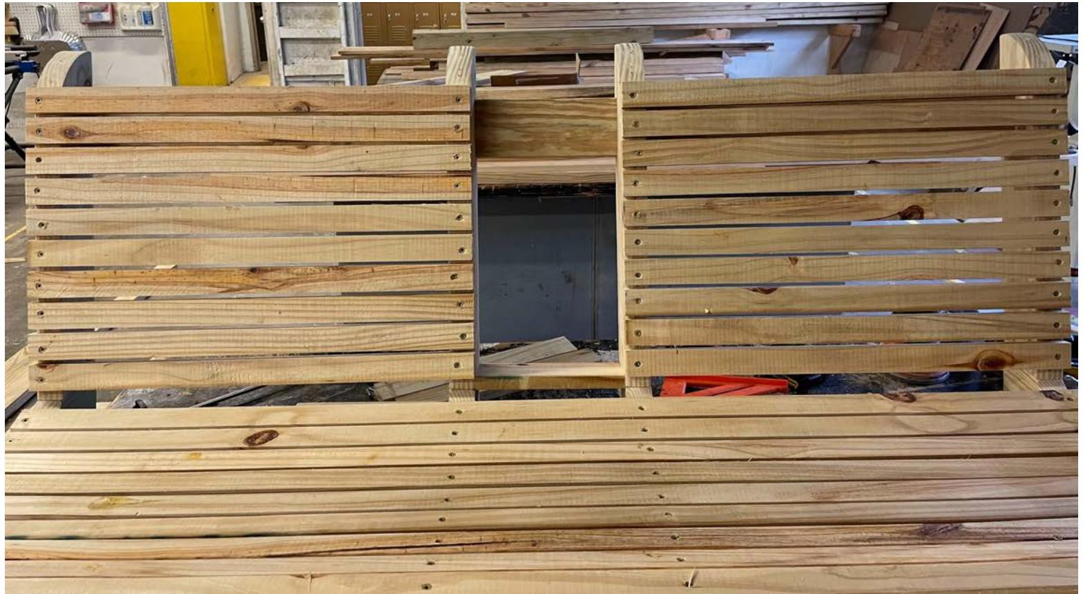
Gap the  $25 \frac{3}{4}$ " back slats  $\frac{1}{4}$ " and install all slats to the back braces using  $1 \frac{1}{2}$ " screws. We recommend pre-drilling holes for the screws to avoid splitting the slats.
