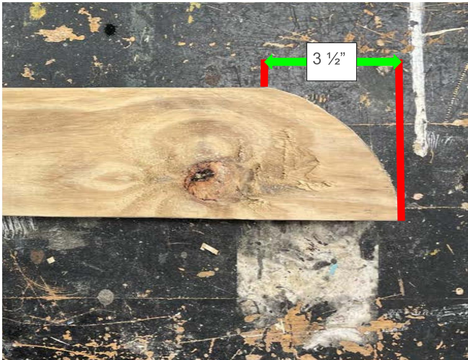
Measure  $3 \frac{1}{2}$ " from the other end of the board and draw a curve from the bottom corner to the  $3 \frac{1}{2}$ " mark then cut out the curve on all 21" and 24" braces.
