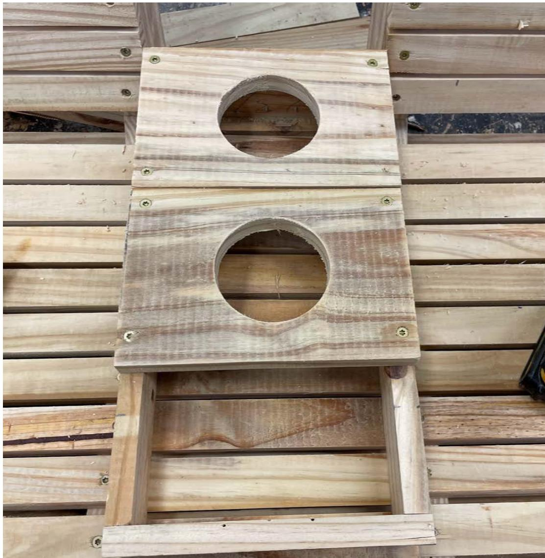
Install the 2 cup holders on the frame from the back and secure with 1  $\frac{1}{2}$ " screws.
