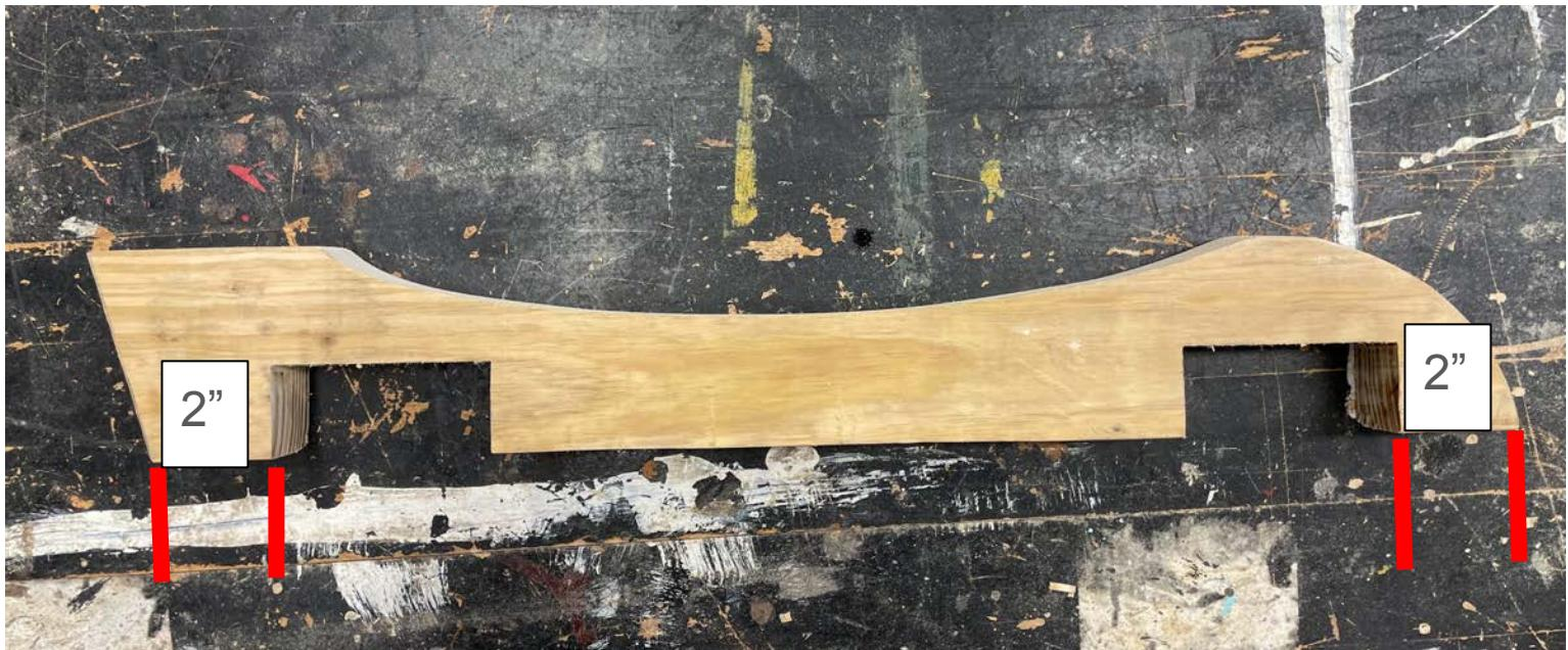
Take 2 of the 24" seat braces and measure 2" from the front and the bottom of the angled end of the braces and cut out the cross brace slats to fit the dimensions of a 2x4 which is  $1\frac{1}{2}'' \times 3\frac{1}{2}''$ .
