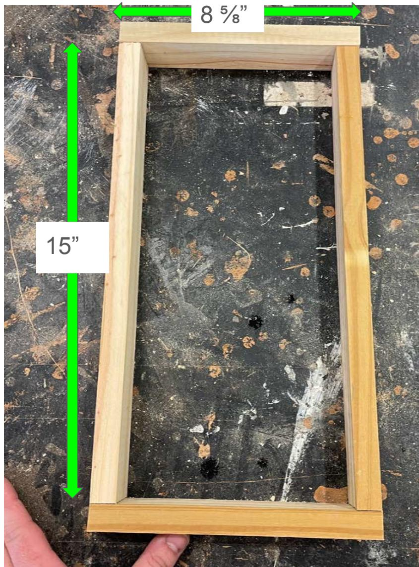
Take your 8' pre-ripped 2" wide strip and cut two 15" pieces and 8  $\frac{5}{8}$ " pieces. Then attach using 1  $\frac{1}{2}$ " screws into a frame.
