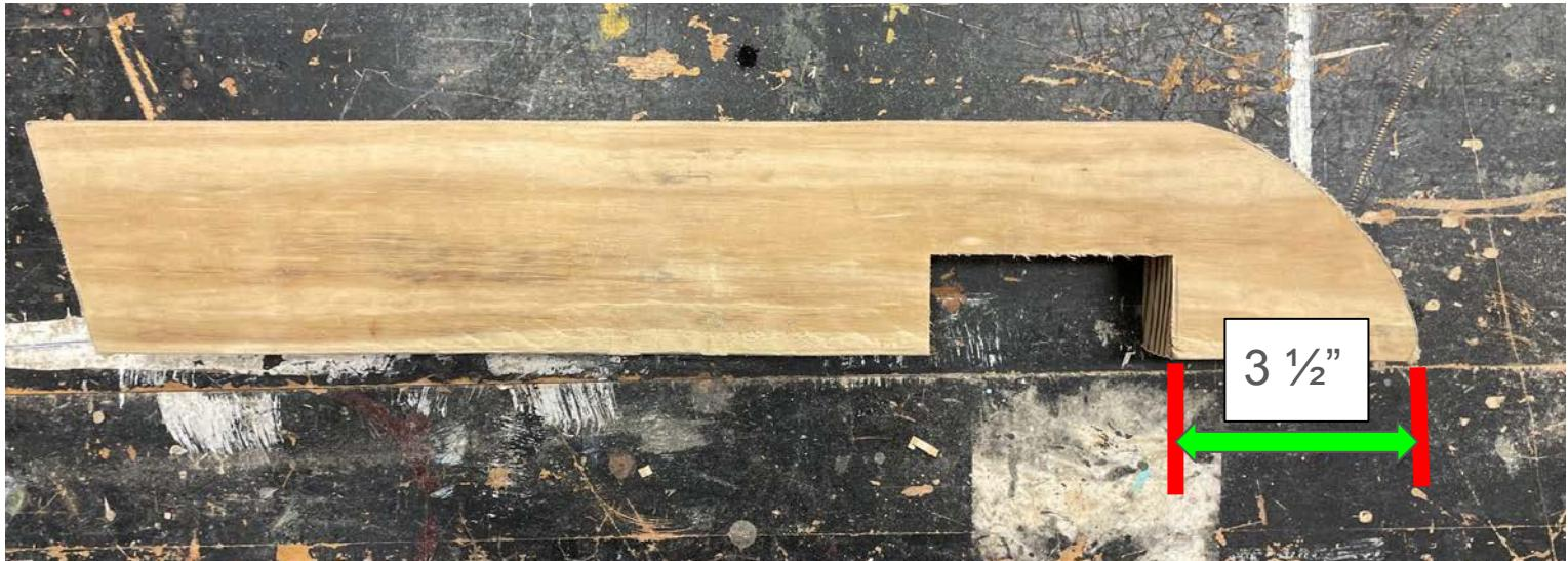
Take two of the 21" back braces and come down 3 ½" from the top of the brace and cut a slat for the swings cross braces. The slat for the brace should be the dimensions of a 2x4 which is 1 ½" x 3 ½".
