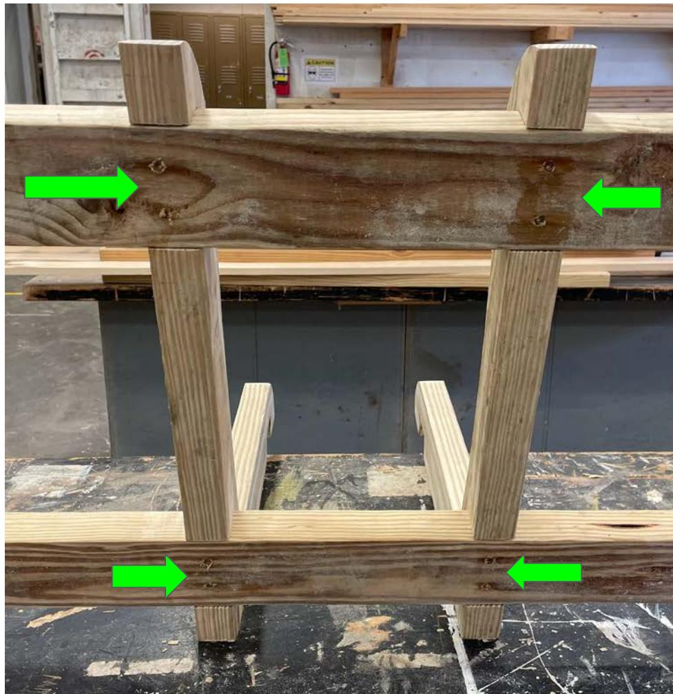
Then flip over and attach the middle braces to the bottom cross braces using 2 1/2" screws
