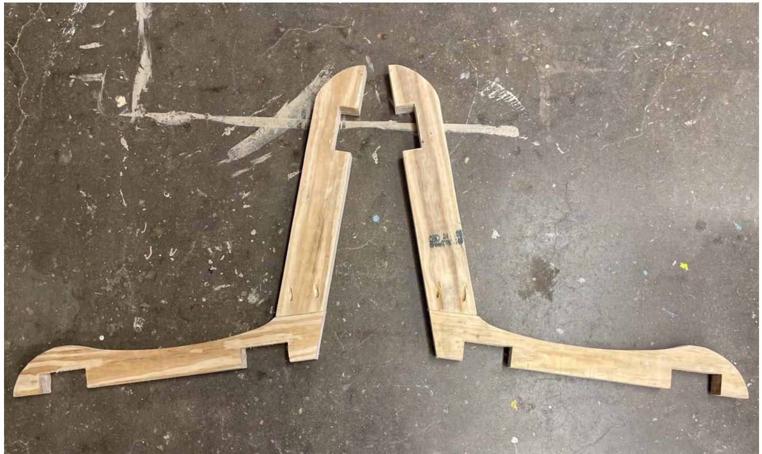
The braces with slats cut out should be attached together while the non slated braces should be attached together.
