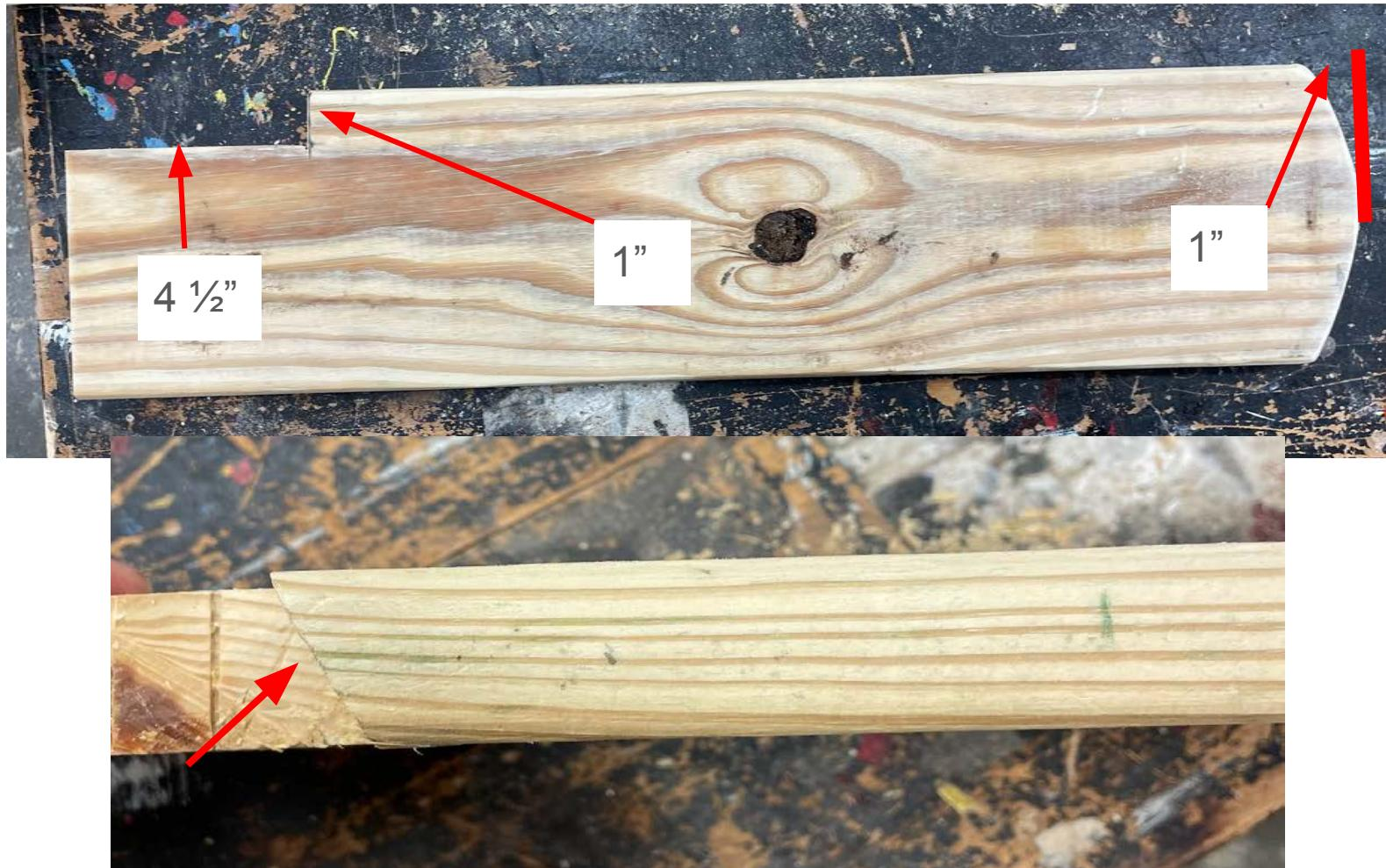
Start by cutting two 24" pieces out of the decking board.
