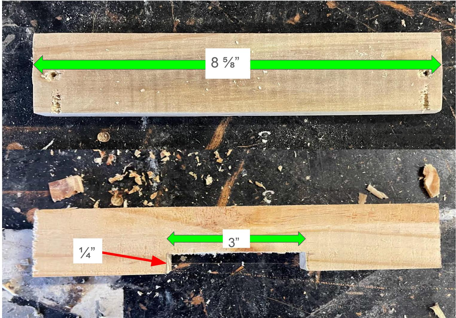
From the pre-ripped 1x2s cut ten  $8 \frac{5}{8}$ " slats for the front of the console. Take one of them and notch a  $\frac{3}{8}$ " x 3" slot. This slat will be the slat that goes over the hinge of the console as the first slat from the bottom.
