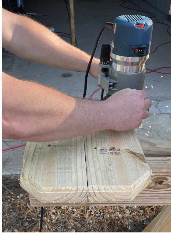
Finally, round off the edges of the table and seats using a router.
