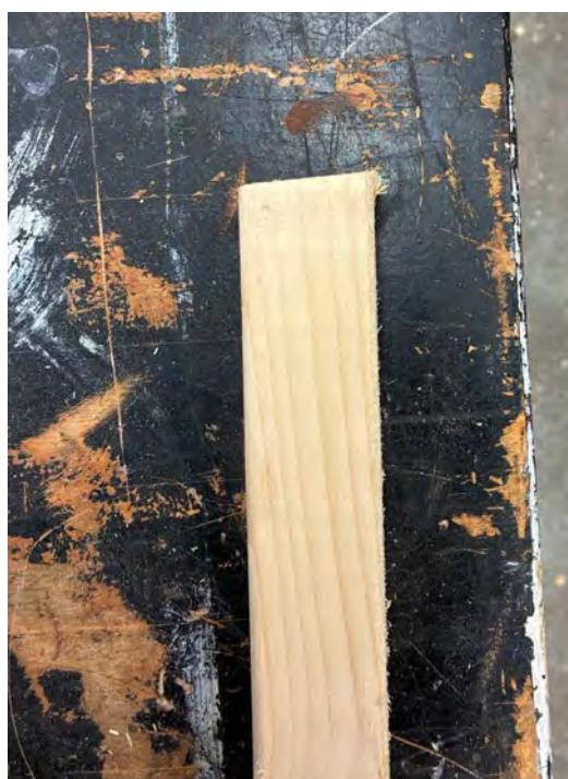
The Top plate for both walls is a 45  $\frac{3}{8}$ " long piece of 2x2 that has 5 degree same angles cut on each end.
