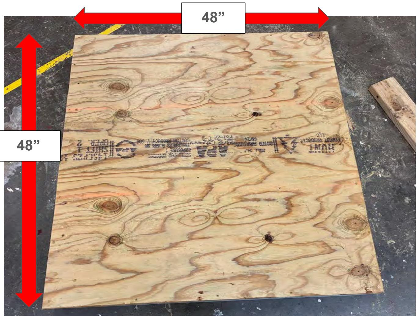
First, cut a 48"x48" piece out of the treated  $\frac{3}{4}$ " plywood sheet.
