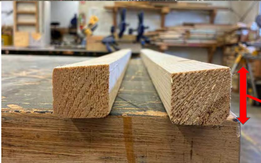
At your Ag Department cut 2 pieces of 2x2 lumber 48" long. Then rip a 5 degree angle on one side of each piece keeping the original 1 1/2" dimension of the board on one side.
