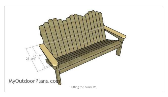
Use 2×4 lumber for the armrests, as well. Fit the armrests to the bench frame, as shown in the diagram. Align everything with attention, and use 2 1/2" screws" screws to lock the components into place. Add glue to enhance the rigidity of the bond.
