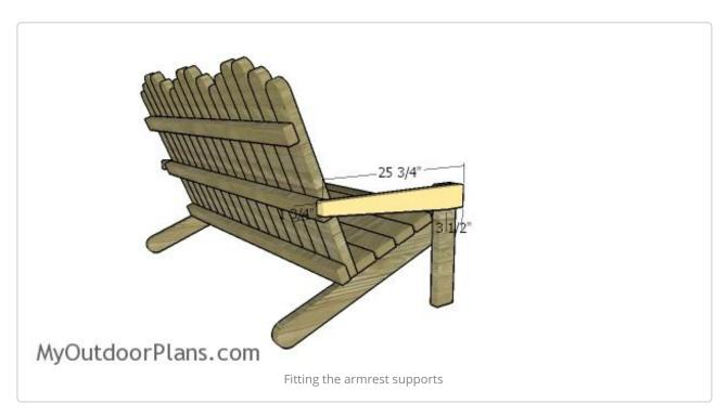
Build the armrest supports from 2×4 lumber. Attach the support to the front legs and to the backrest of the chair. Drill pilot holes and insert 2 1/2" screws to lock the support into place. Leave no gaps between the components and make sure the edges are perfectly aligned.
