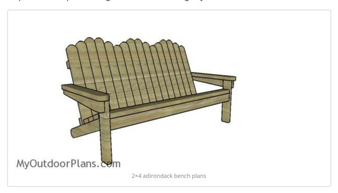
Fill the holes with wood putty and let them dry out for a few hours. Smooth the surface with 100-200 grit sandpaper and remove the residues with a damp cloth. Apply a few coats of stain or paint to enhance the look of the chair.
