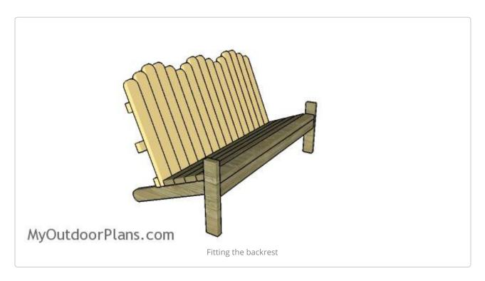
Attach the backrest to the frame of the bench. Drill pilot holes through the bottom support of the backrest into the back legs. Make sure the backrest makes a 90 degree angle with the seat.
