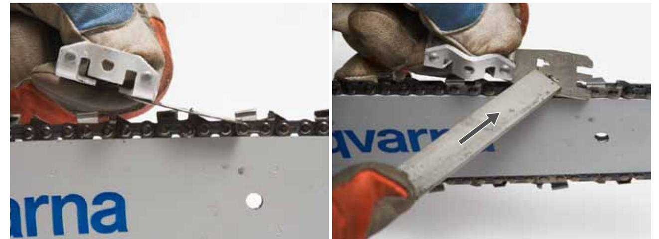
1. Add the gauge and hold it firmly with one hand. Select “Soft” or “Hard”, depending on the wood you are sawing. The depth gauge varies with the type of chain.
