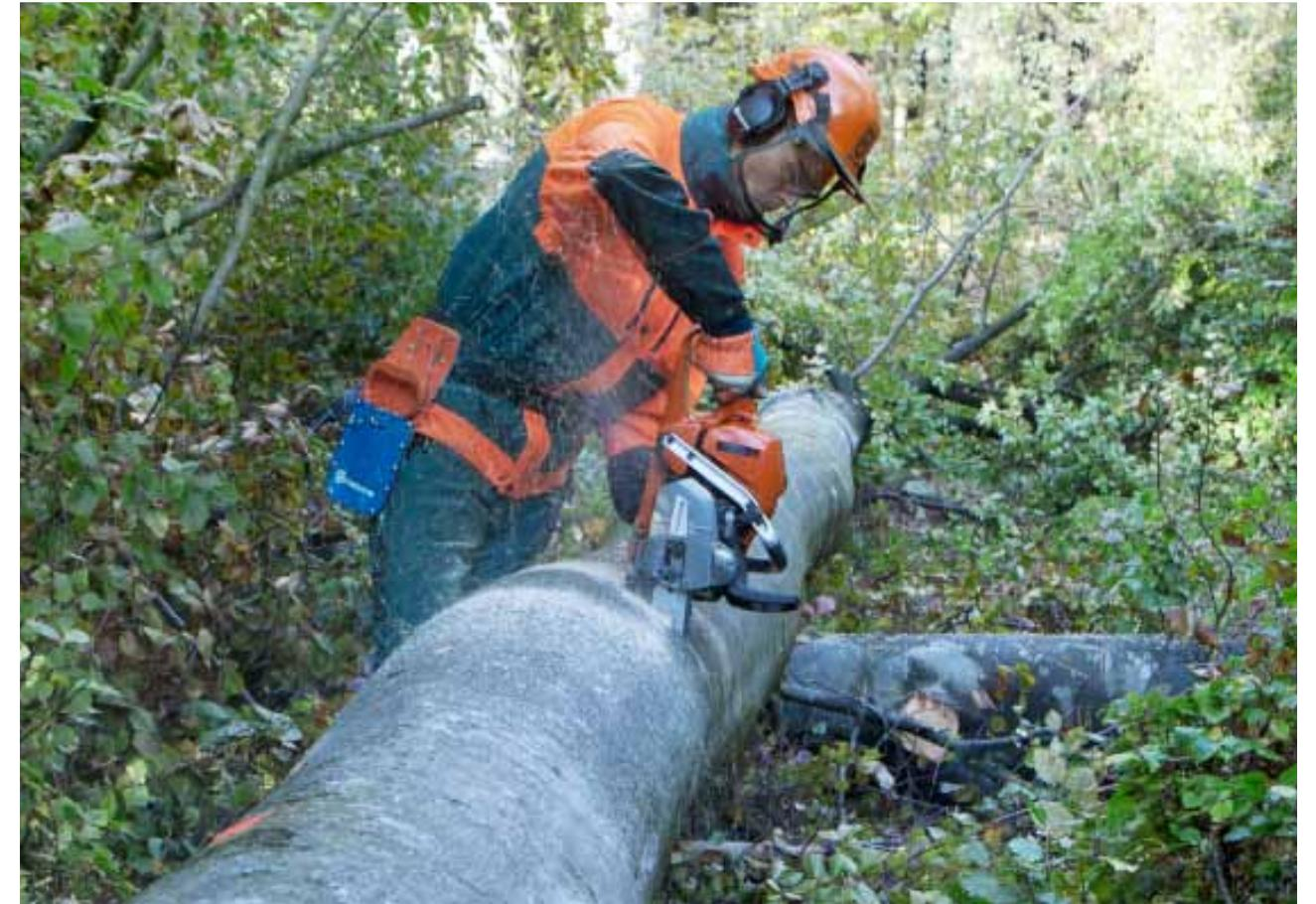
**If the trunk is thicker than the guide bar length.**
