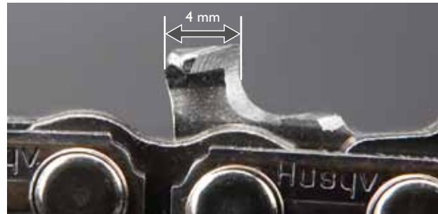
*Over-sharpened cutting tooth. If the cutting tooth is shorter than 4 mm, the chain must be discarded.*
